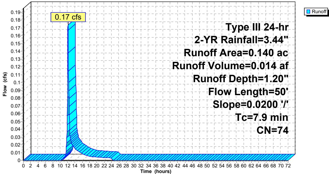
**Hydrograph for Subcatchment 9: A2 ON-SITE (PERV)**
