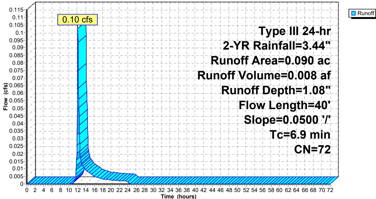
**Hydrograph for Subcatchment 11: A3 ON-SITE (PERV)**
