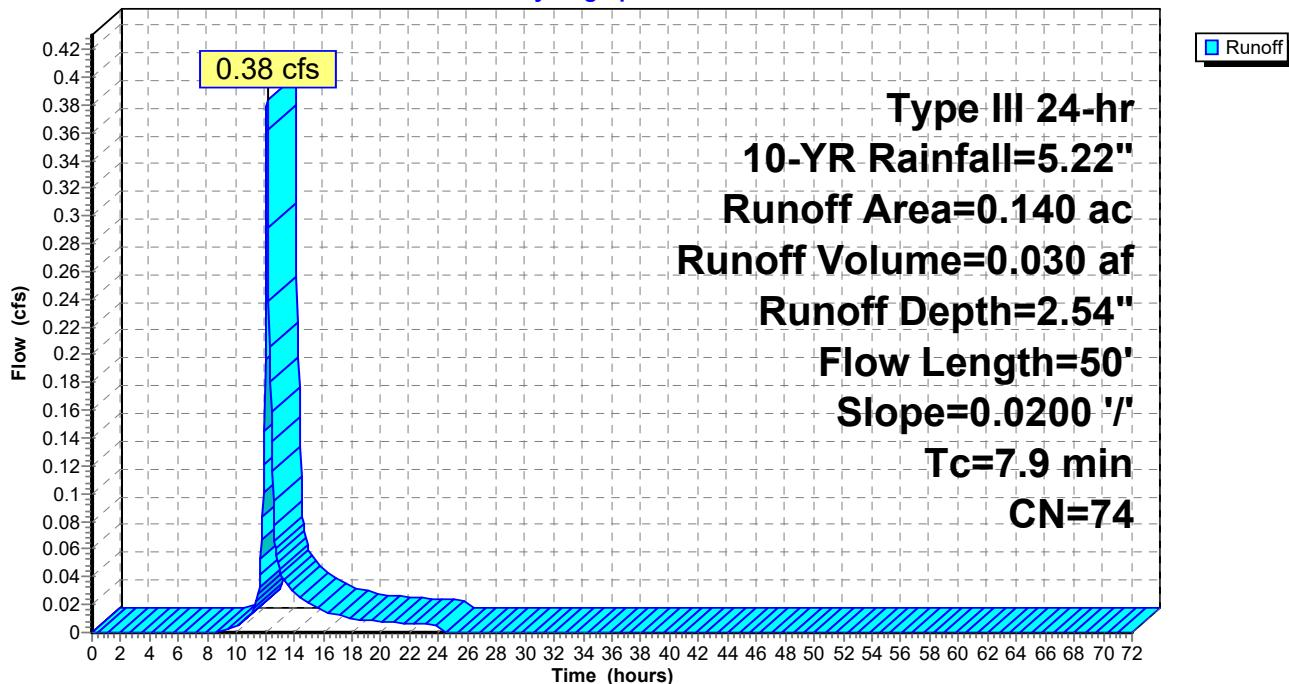
**Hydrograph for Subcatchment 9: A2 ON-SITE (PERV)**
