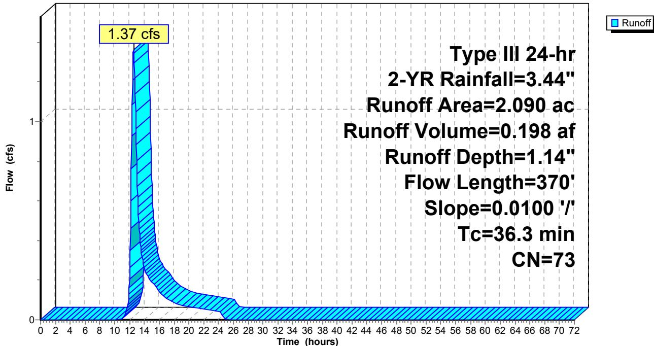
**Hydrograph for Subcatchment 2: A1 ON-SITE (PERV)**
