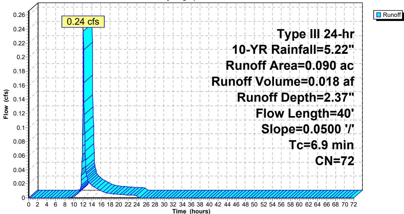
**Hydrograph for Subcatchment 11: A3 ON-SITE (PERV)**
